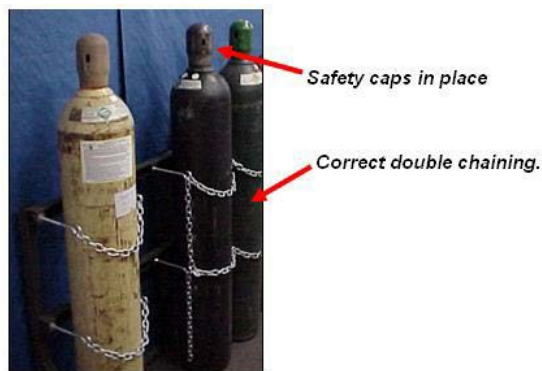
Figure 2. Correct cylinder storage
