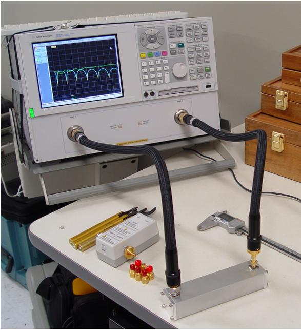
a) Network Analyzer and Waveguide
