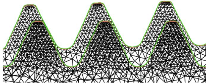
Distorted mesh (with a scale factor of 10) after the cooling stage.
