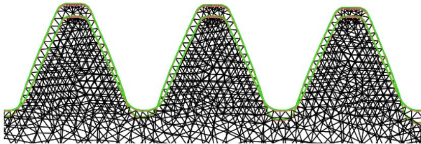
Distorted mesh (with a scale factor of 10) after the heating stage.
