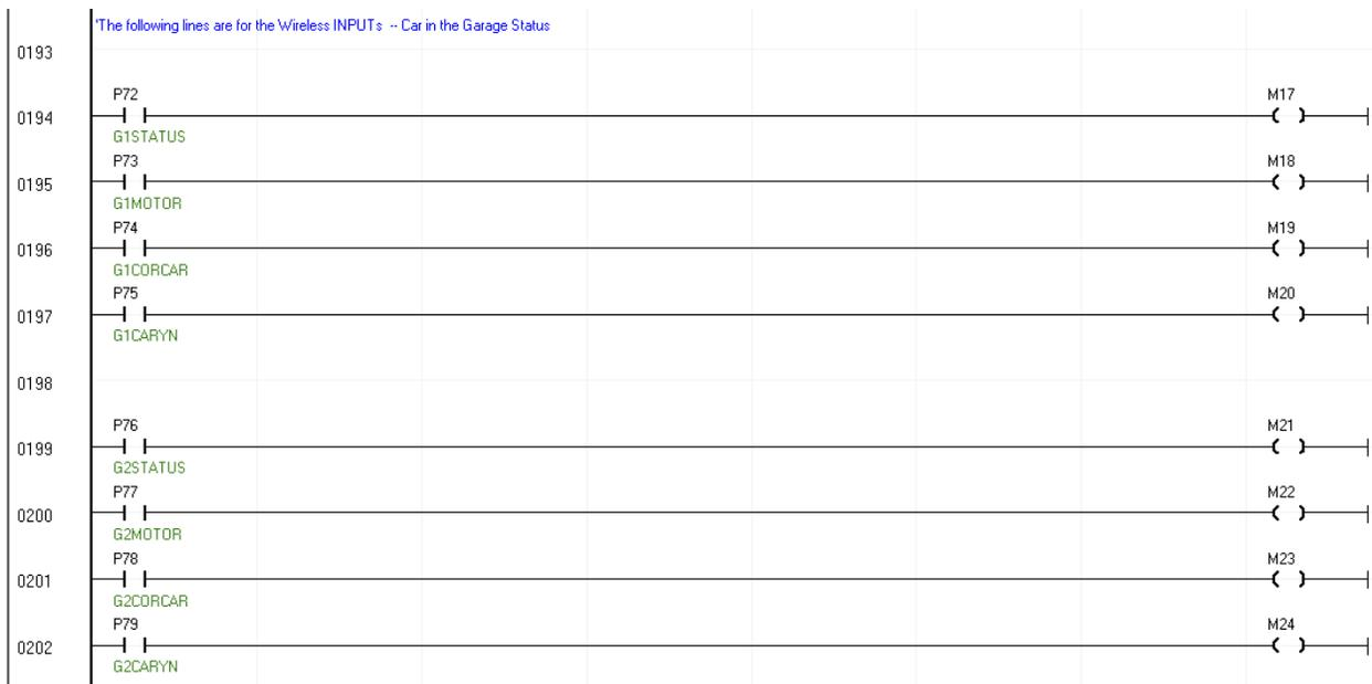
Figure 5.6 PLC Logic for Car in the Garage Status
