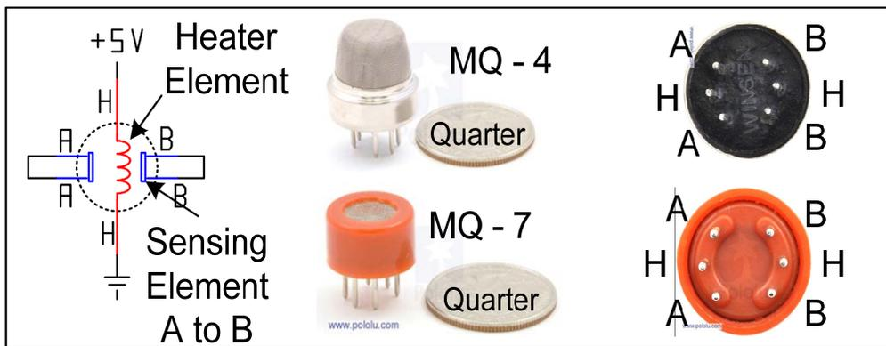
Figure 4.5 Typical MQ Series Gas Sensors
