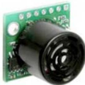
Figure 4.3 Maxbotix MB1010 Sonar Range Finder Sensor
