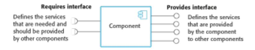
Note UML notation. Ball and sockets can fit together.
