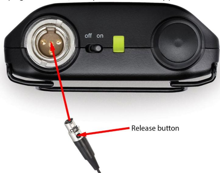
3. Align the pins on the plug with the pins on the mic pack and insert until fully seated.
