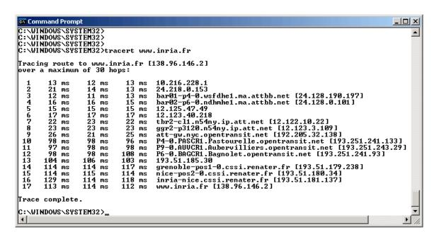
**Figure 4** Command Prompt window displays the results of the Traceroute program.
