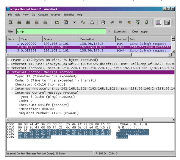
Figure 5 Wireshark window of ICMP fields expanded for one ICMP error packet.
