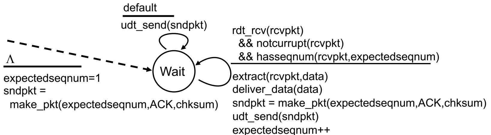
ACK-only: always send ACK for correctly-received
