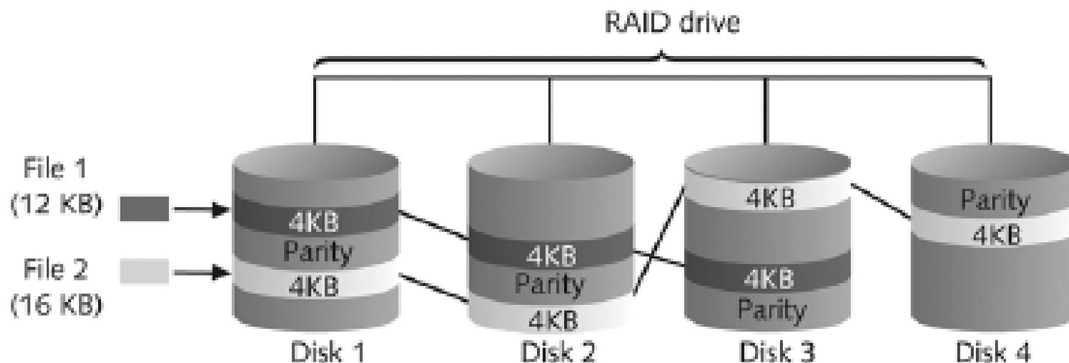
Figure 4-14 RAID 5: Block-level striping with distributed parity
