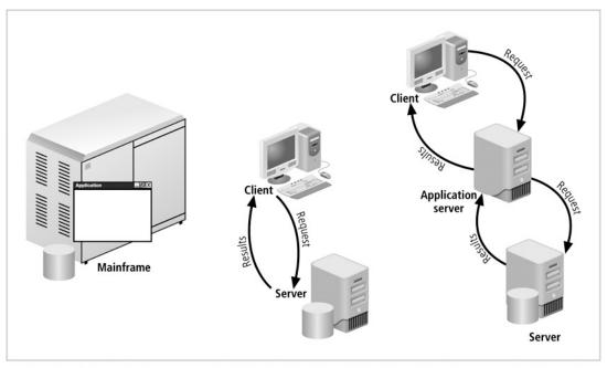
FIGURE 1-3 Examples of different client/server tier design
