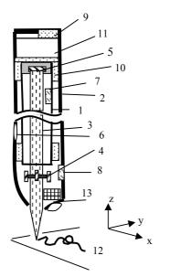
Figure 1. Block scheme of the BiSP device for data acquisition. (1) inner case (2) outer case (3) refill (4) x,ypressure sensors (5) z-pressure and vibration sensor (6) fingerprint chip (7, 8) inner, outer microphone (9) loudspeaker (10) acoustic isolation placed between the cases (11) electronics and data storage (12) ink trail on normal paper (13) optical sensors.
