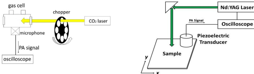
**PROJECT 1:** Photoacoustic spectroscopy will be used to test the photoacoustic properties of an optically thick and potent greenhouse gas. Detection of trace amounts of the gas is also implemented. The conditions in which the gas is tested, gas cell length, temperature, concentration, and power of the laser, will be varied in order to determine their effect on the photoacoustic signal, and an ideal condition to detect trace gas amounts. A detection limit will be determined for greenhouse gas.
