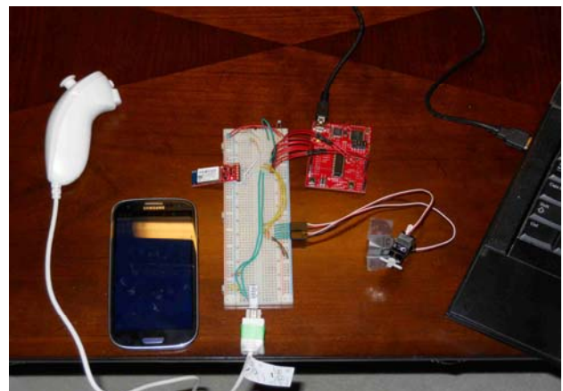
Fig. 1. Android external vibration sensory embedded system with Bluetooth
