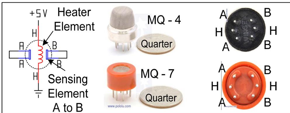
Figure 4.5 Typical MQ Series Gas Sensors
