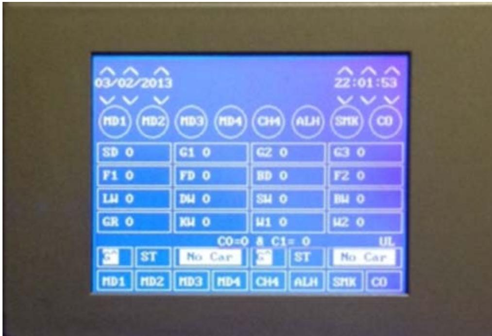
Figure 6.1 The HMI Touch Screen Interface
