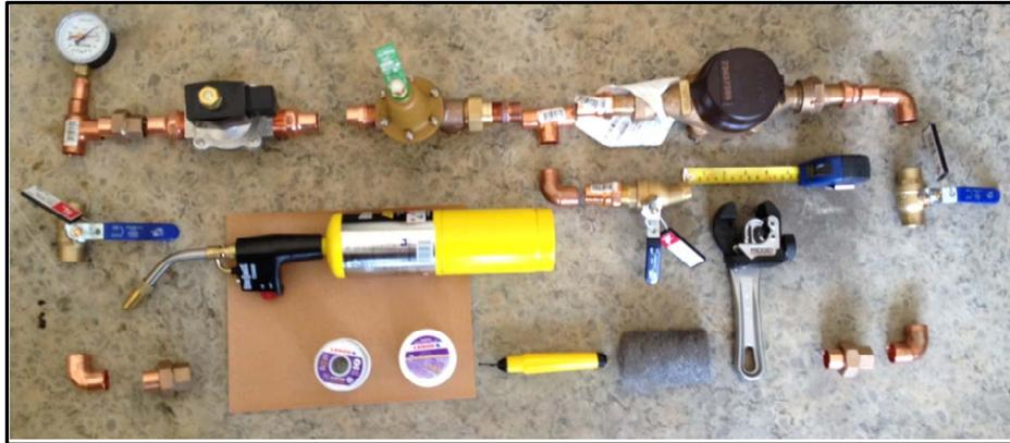
Figure 3.6 Items Needed for the Water Meter and Electric Shut-Off Valve Installation
