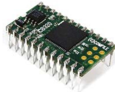
Figure 4.9 CB320 Microprocessor and PLC on a Chip
