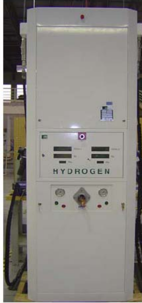
Figure 5: Photograph of a hydrogen dispensing unit.
