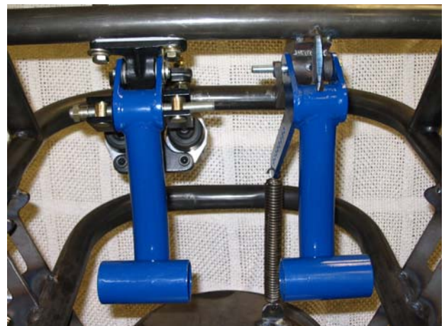
Figure 10. Brake System mounted on Chassis.
